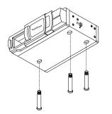
Save the shipping screws in case you might want to install the CD changer in another vehicle. You can secure them to the back of the CD changer with a piece of tape.
